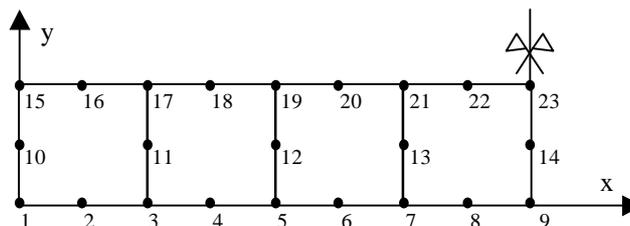
Figure 2 – Mesh, four eight-node elements
