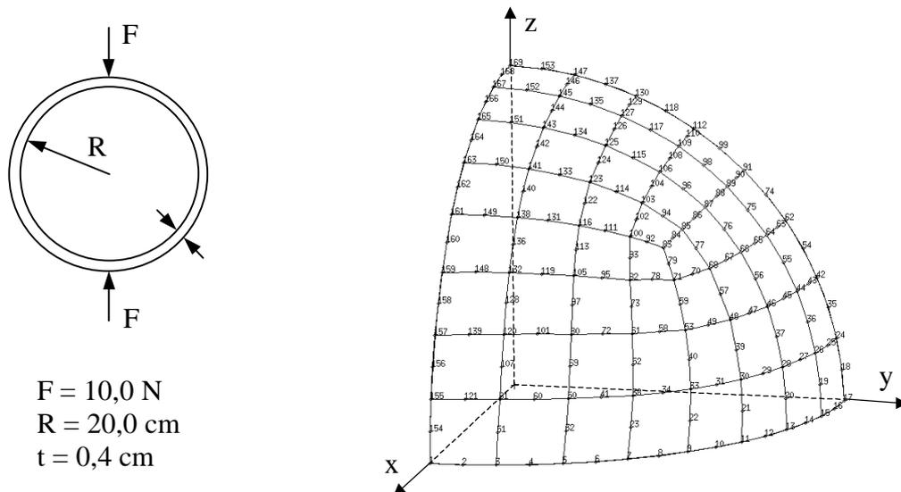
Figure 6 – Load configuration, geometry and used mesh
