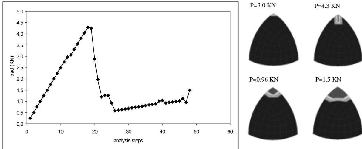
Figure 7 – Load-time variation and failure configurations
