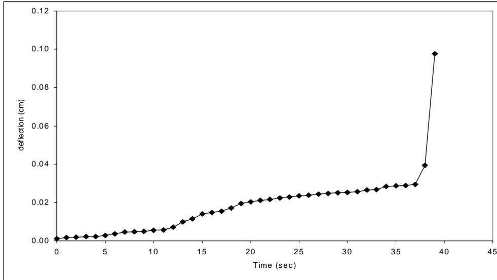
Figure 5 – Deflection-time plot for viscoelastic failure analysis in buckling
